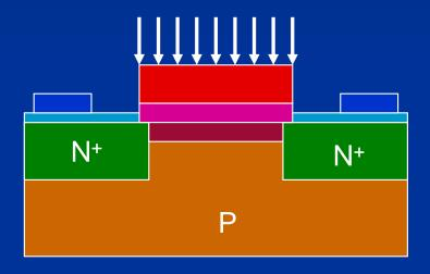
Low K<sub>gate</sub> Larger I<sub>gate</sub>, Smaller delay
