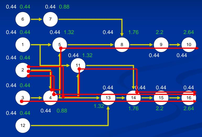
Network with Path Delays (Fix,  $D_T = 2.64$ )
