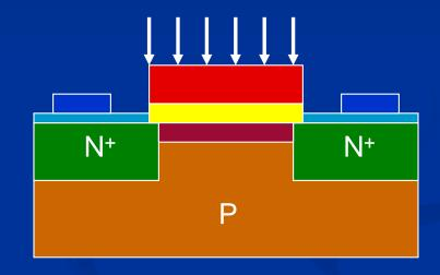
High K<sub>gate</sub> Smaller I<sub>gate</sub>, Larger delay
