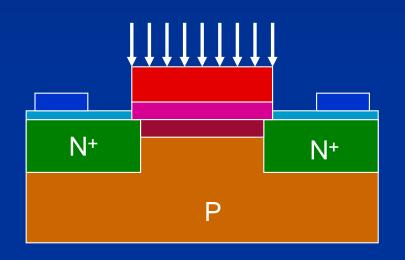
Low T<sub>gate</sub> Larger I<sub>gate</sub>, Smaller delay
