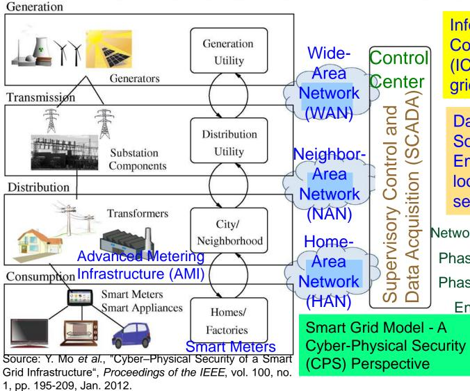
Information and Communication Technology (ICT) components of smart grid is cyber vulnerable.
