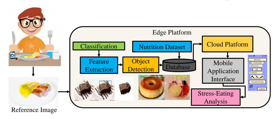
iLog-Fully Automated Detection System with 98% accuracy.
