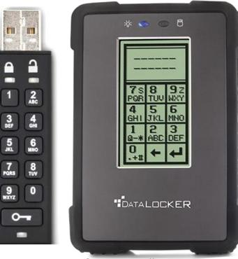
Source: http://datalocker.com Nonvolatile / Harddrive Storage Hardware-based encryption of data secured/protected by strong password/PIN authentication.
