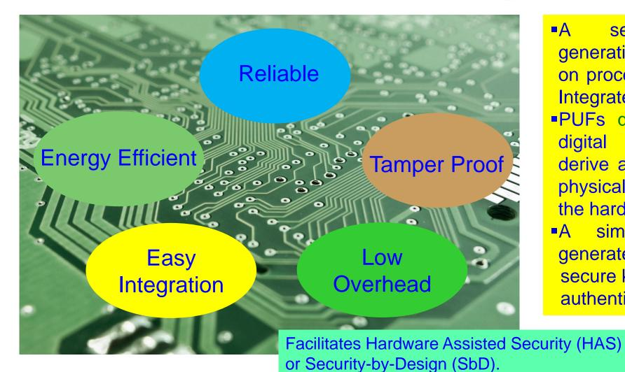
fingerprint ■A secure generation scheme based on process variations in an **Integrated Circuit** PUFs don't store keys in memory, digital rather derive a key based on the physical characteristics of the hardware; thus secure. A simple design that generates cryptographically secure keys for the device authentication
