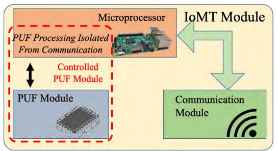
Source: V. P. Yanambaka, **S. P. Mohanty**, E. Kougianos, B. K. Baniya, and B. Rout, "<u>Veda-PUF: A PUF based on Vedic Principles for Robust Lightweight</u> <u>Security for IoT</u>", in *Proceedings of the 7th IEEE International Symposium on Smart Electronic Systems (iSES)*, 2021, pp. 400--405, DOI: <u>https://doi.org/10.1109/iSES52644.2021.00097</u>.
