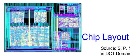
Chip Design Data Total Area : 16.2 sq mm, No. of Transistors: 1.4 million Power Consumption: 0.3 mW, Operating Frequency: 70 MHz and 250 MHz at 1.5 V and 2.5 V
