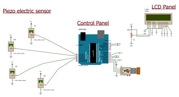
Fig. 4: ARDUINO based sensor module to monitor weight of individual box elements.
