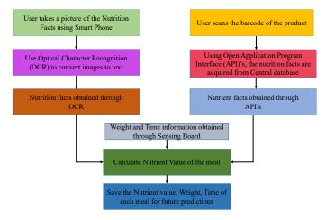
Fig. 2: Flow chart of data acquisition involved in the nutrition monitoring system.
