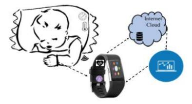
Fig. 1: Basic Architecture of Smart-Pillow System.
