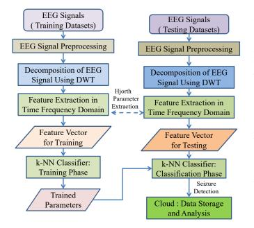
Fig. 3: Flowchart of the proposed novel fast and accurate seizure detection algorithm.
