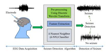
Fig. 1: Block diagram of the proposed seizure detection paradigm.
