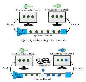
Fig. 4: Impact of eavesdropping on a quantum channel.
