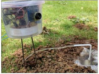
(b) Less soil moisture level, prototype setup with irrigation.Fig. 12: IoAT Experimental Prototype.
