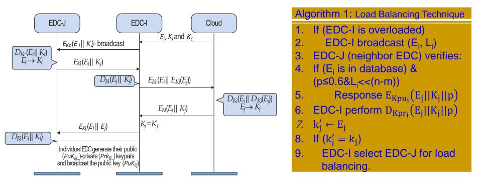
Secure edge datacenter – ➤ Balances load among the EDCs ➤ Authenticates EDCs Response time of the destination EDC has reduced by 20-30% using the proposed allocation approach.
