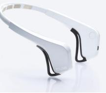
Headband with Embedded Neurosensors
