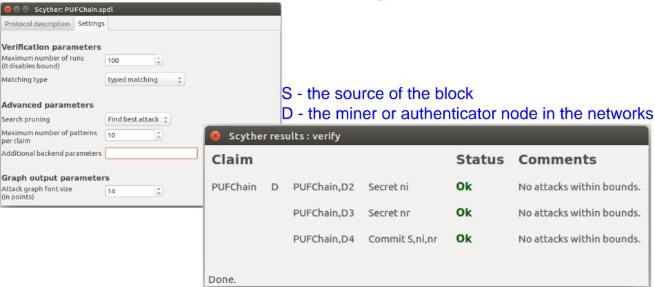
PUFchain Security Verification in Scyther simulation environment proves that PUFChain is secure against potential network threats.
