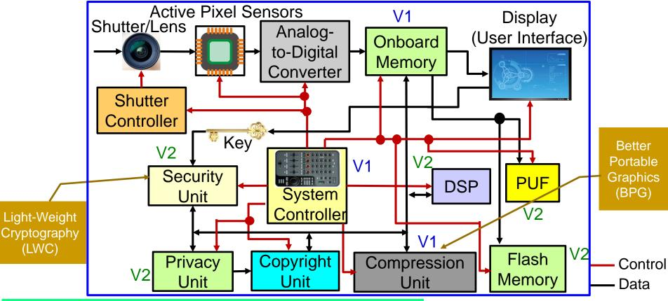
Include additional/alternative hardware/software components and uses DVFS like technology for energy and performance optimization.
