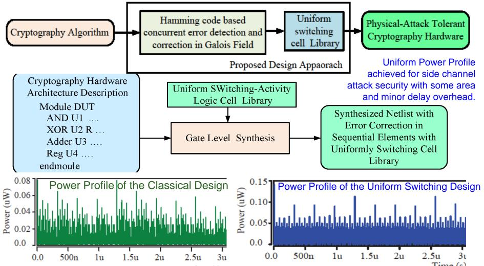
Source: J. Mathew, S. P. Mohanty, S. Banerjee, D. K. Pradhan, and A. M. Jabir, "Attack Tolerant Cryptographic Hardware Design by Combining Galois Field Error Correction and Uniform Switching Activity", *Elsevier Computers and Electrical Engineering*, Vol. 39, No. 4, May 2013, pp. 1077--1087.
