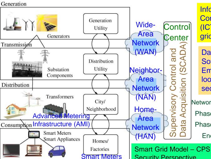
Information and Communication Technology (ICT) components of smart grid is cyber vulnerable.
