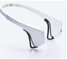
Headband with Embedded Neurosensors
