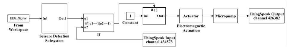
• Upon seizure detection, the drug delivery unit becomes active and the coil acts as an electromagnet.
