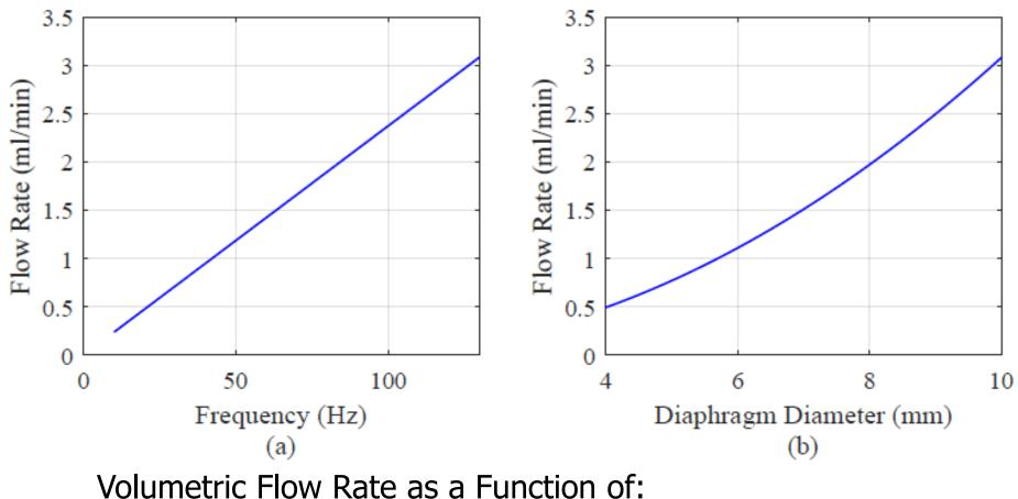
(a) Actuation Frequency (b) Diaphragm Diameter.
