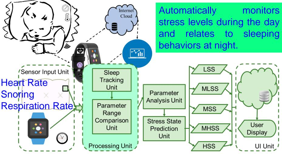
Source: Mohanty iSES 2018: "Smart-Pillow: An IoT based Device for Stress Detection Considering Sleeping Habits", in *Proc. of 4th IEEE International Symposium on Smart Electronic Systems (iSES)* 2018.
