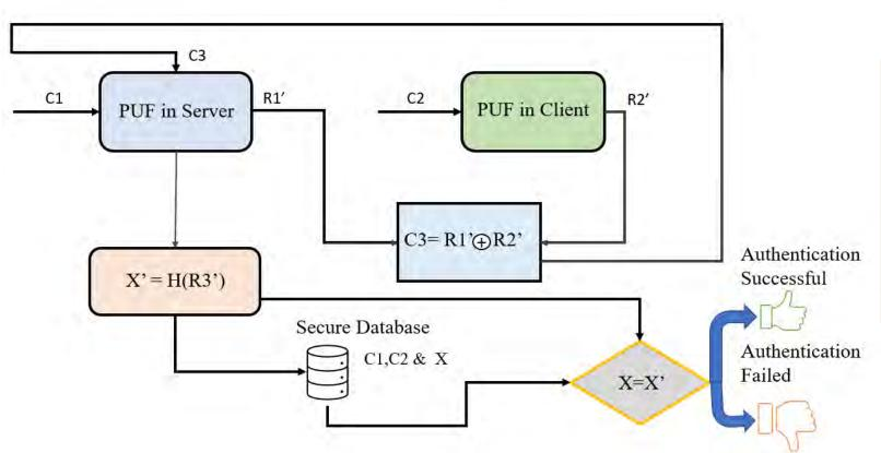
Only C1 and C2 are retrieved and given as inputs to the PUF module. The final Hash value X is compared with the stored hash value X to authenticate the device
