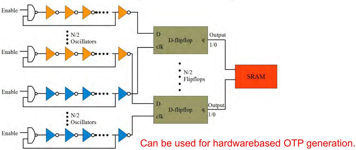
Source: V. P. Yanambaka, **S. P. Mohanty**, E. Kougianos, and J. Singh, "<u>Secure Multi-Key Generation Using Ring Oscillator based Physical Unclonable</u> <u>Function</u>", in *Proceedings of the 2nd IEEE International Symposium on Nanoelectronic and Information Systems (iNIS)*, 2016, pp. 200--205.
