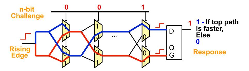
Compare two paths with an identical delay in design – Random process variation determines which path is faster – An arbiter outputs 1-bit digital response
