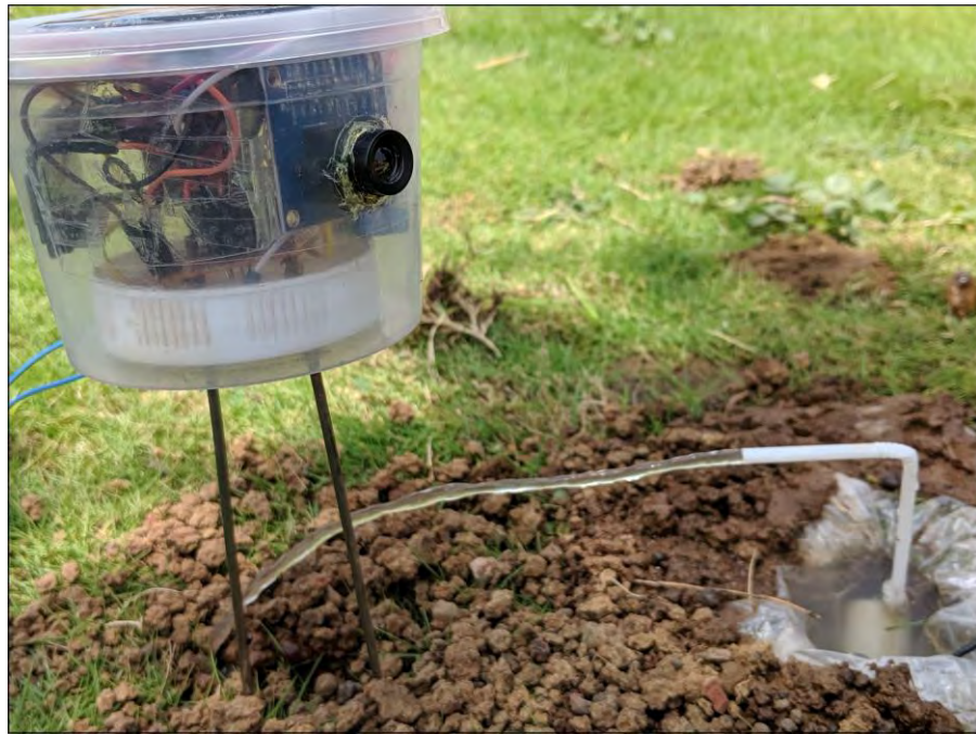
sCrop Device Prototype with Irrigation
