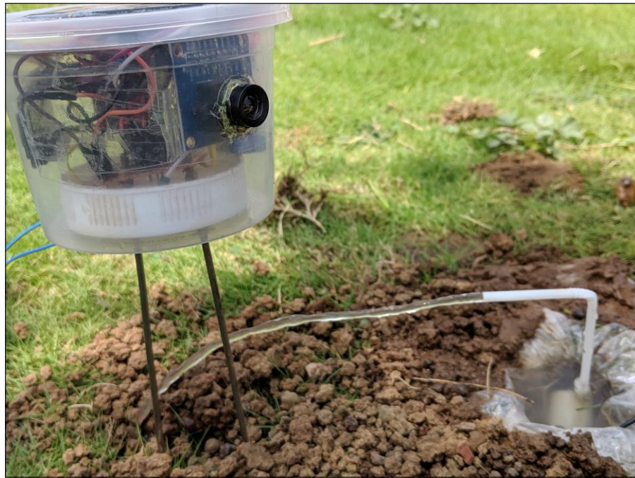
sCrop Device Prototype with Irrigation
