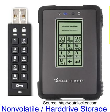
Hardware-based encryption of data secured/protected by strong password/PIN authentication.
