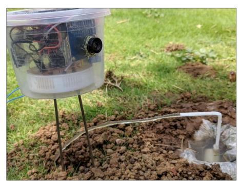
sCrop Device Prototype with Irrigation
