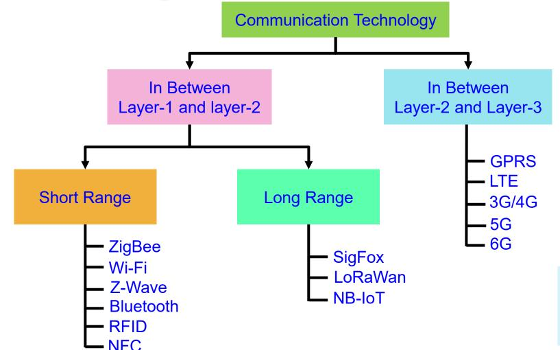
Connectivity Layer-1: Near Range ZigBee, Wi-Fi, Z-Wave, Bluetooth, Radio Frequency Identification (RFID), and Near Field Communication (NFC).
