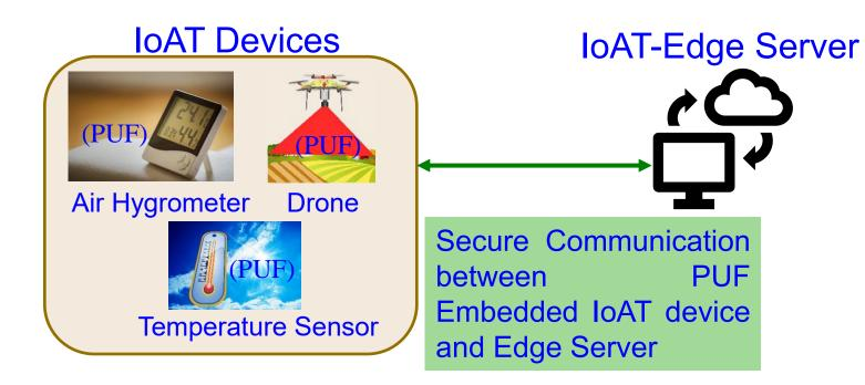
Edge Server authenticates the devices using the PUF key of each electronic device which is the fingerprint for that device
